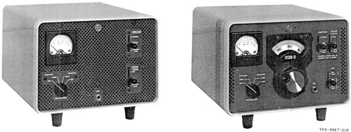
Figure 1. 312B-4 and 312B-5 Station Controls
