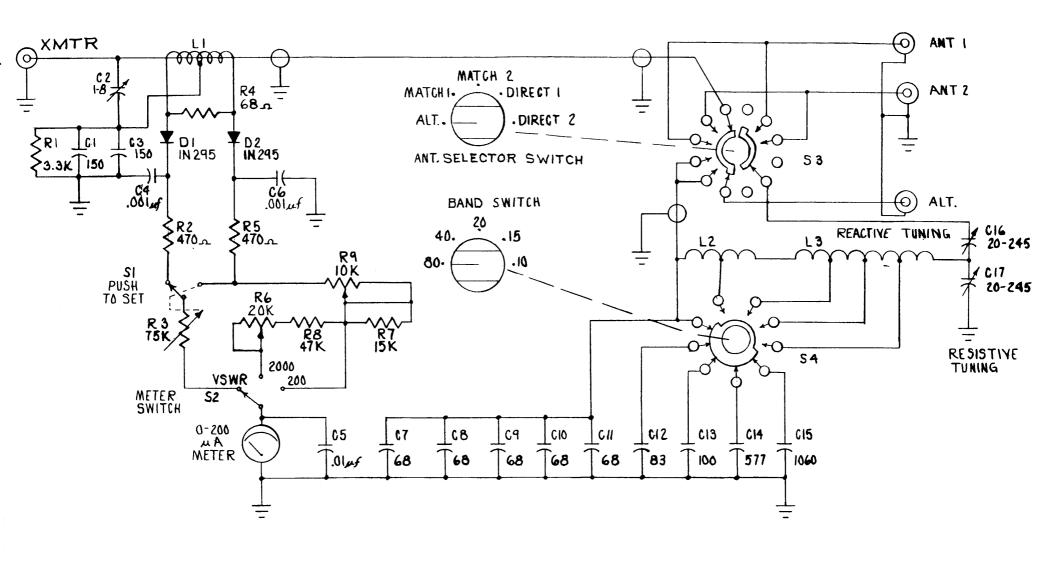
Figure 4-1. Model MN-2000 Matching Network Schematic Diagram
