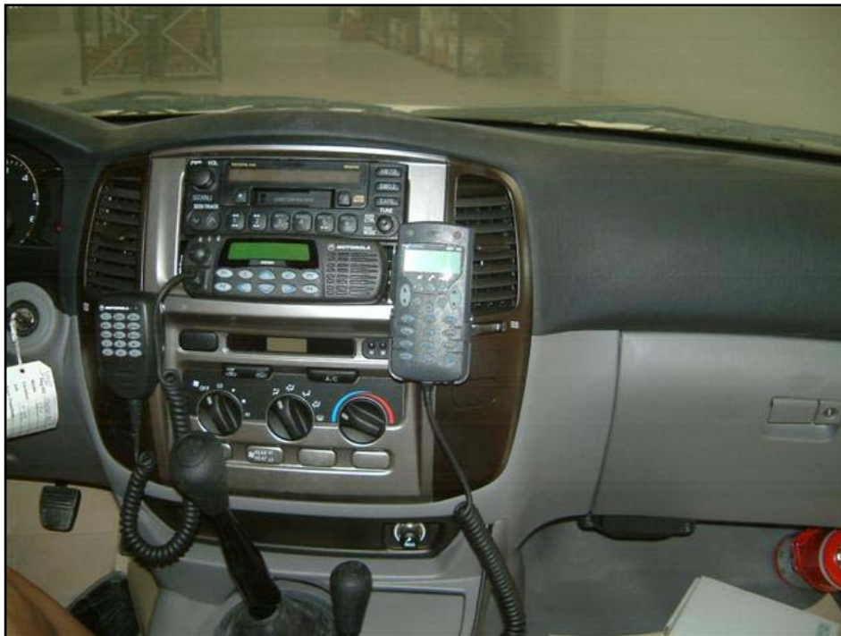
Typical installation of mobile radios in Toyota L/C
