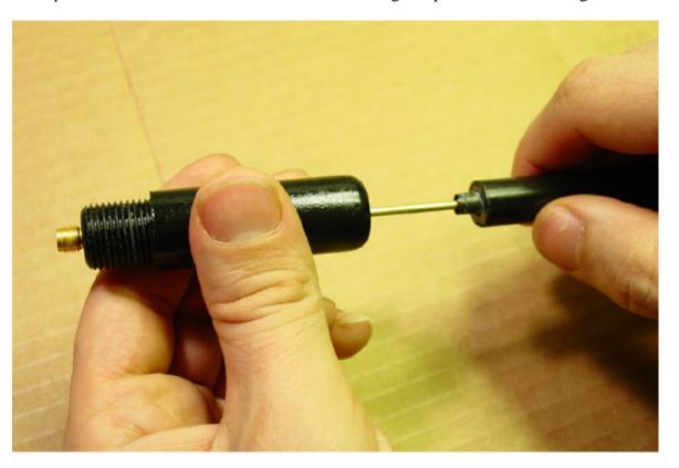
Figure 16. Retracting the radome once decoupler is set.
