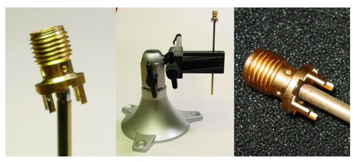
Figure 5: The image on the left shows the solder applied to the center conductor now resting on the feed prior to feedline heating. The center image shows the feedline in vise, after heating the tube and allowing the connector to rest flat on the top of the feedline tube. The image on the right shows the completed feedline soldered to SMA center conductor.
