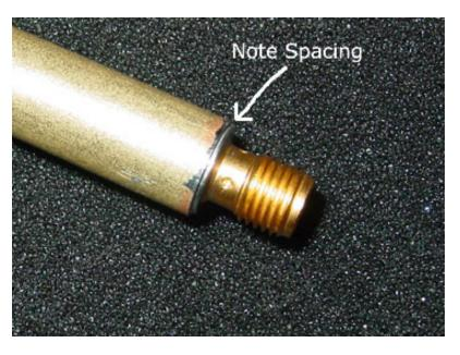
Figure 6: Decoupling sleeve over SMA connector. Note minimal spacing between SMA base and edge of decoupler sleeve.
