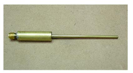
Figure 7: Completed decoupler assembly.
