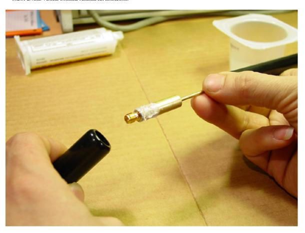
Figure 14. Epoxy applied to decoupler and about to be aligned into the threaded mounting component.
