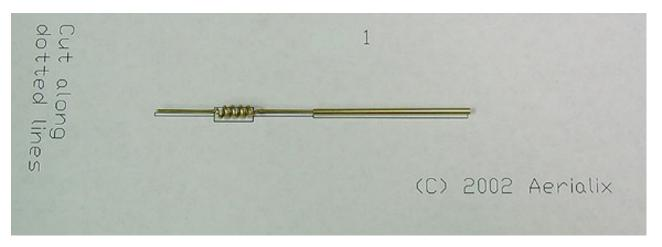
Figure 9. Aligning an element assembly using template T1 as a guide.
