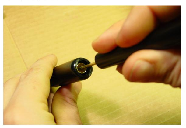
Figure 15. Aligning the decoupler in the threaded mounting component.
