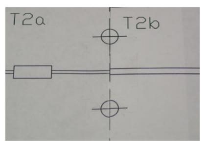
Figure 10. Proper joining of template T2a and T2b.
