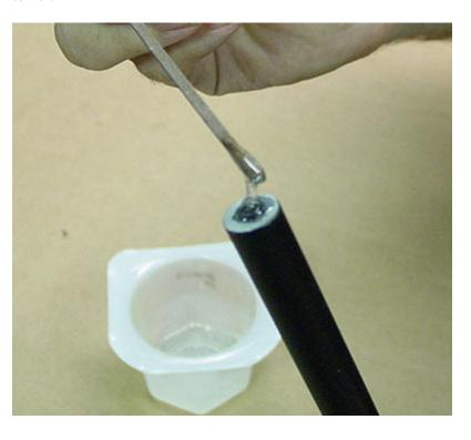
Figure 18. Applying epoxy into the top end of the radome.
