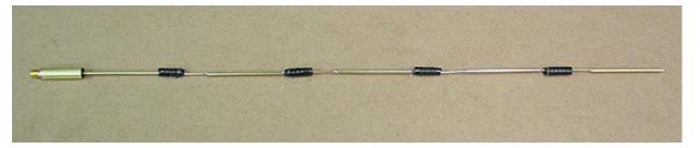
Figure 13. Anti-rattling tape applied to the coils.
