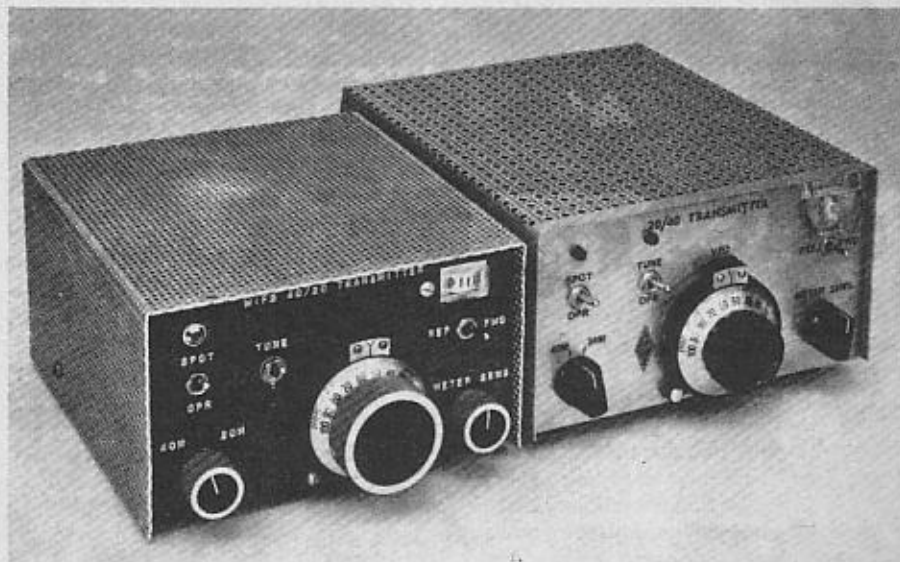
Two versions of the 7- and 14-MHz cw transmitter are shown here. At the left is the W1FB prototype. On the right is a model built by WA0UZO. Both units are small and lightweight.
