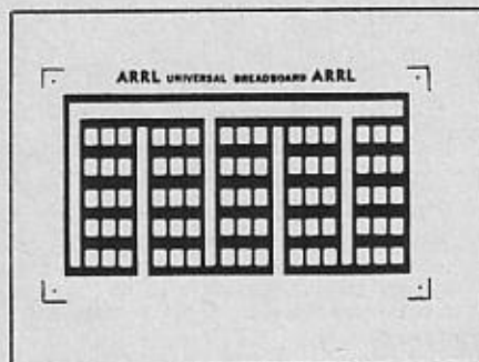
Fig. 5 — Suggested pattern for a universal breadboard that can be etched as shown, not to scale. A +V and a ground bus are provided for easy access along the length of the board. See the "Hints and Kinks" section of this issue for a full-size pattern template.
