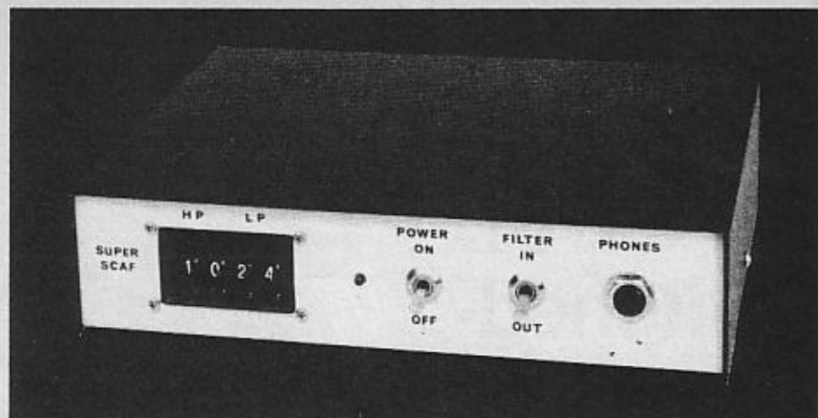
SuperSCAF is a stand-alone unit that contains a switched-capacitor filter, an audio power amplifier and an ac-operated power supply.
