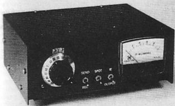
Fig. 47 — The completed 6-W VXO controlled transmitter is housed in a small aluminum enclosure. RG-174 is used for all interconnections carrying RF. This version uses the older MRF472 output transistors, which are mounted flat on the board.
