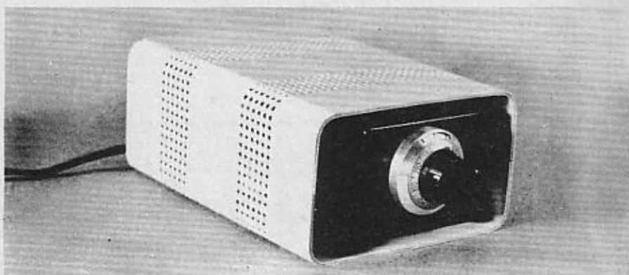
The Vackar oscillator VFO enclosed in an attractive, contemporary-styled cabinet. Below is an inside view showing rather high component density. The U3 output amplifier is on a separate board next to the transformer.
