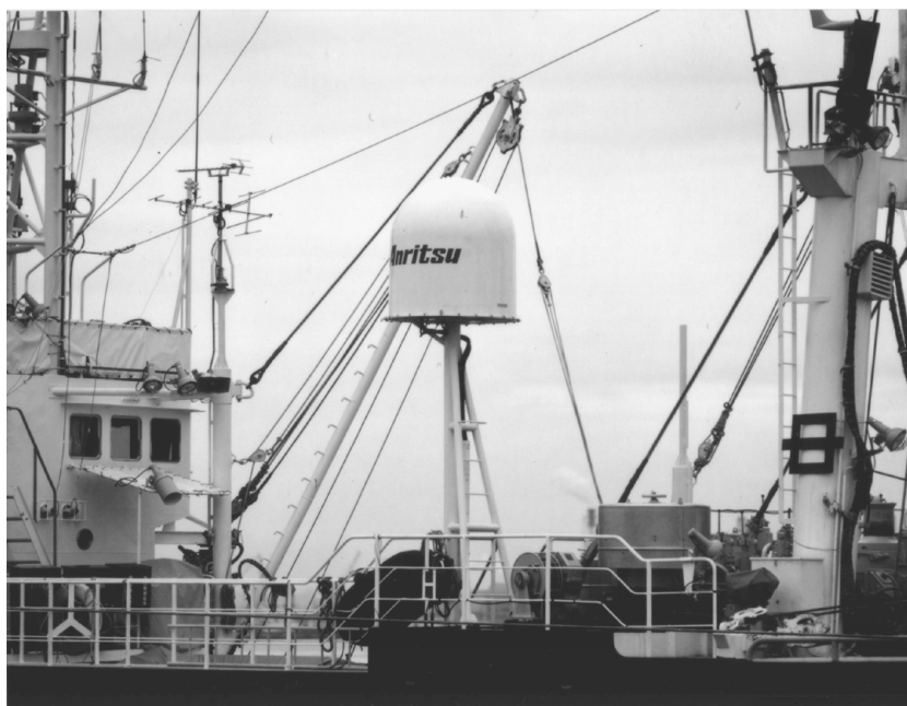
FIGURE 13.2 Photograph of above-deck equipment (ADE) installed on a ship. An antenna unit is covered with a radome. (Courtesy of Anritsu).
