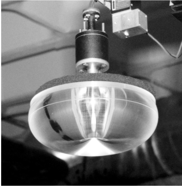
FIGURE 15.27 Prototype of 28\text{-}\lambda lens for \sec^2 \theta coverage of circular cells, at the 60-GHz band. (From Fernandes, C.A., IEEE Antennas Propag. Mag. , 41, 141, 1999. With permission.)
