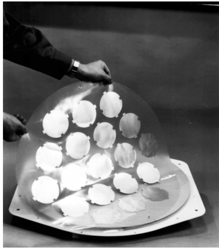
FIGURE 13.18 A 19-element phased-array antenna printed on a very thin film. The G/T is about -13 dBK at an elevation angle of 45^\circ , and the performance was evaluated using the ETS-V satellite and an open-loop tracking method.
