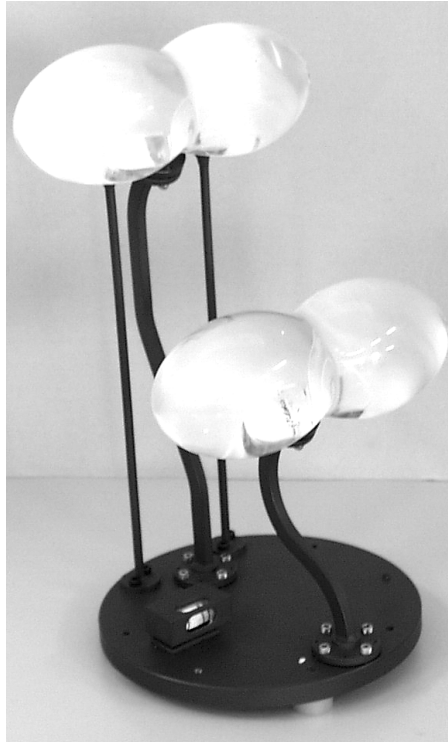
FIGURE 15.39 Lens assembly for elongated cell illumination, 39.5 to 43.5 GHz, G = 14 dBi.
