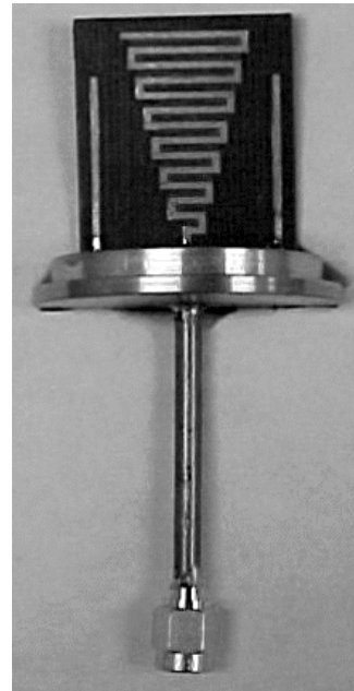
FIGURE 12.44 The prototype of dual-sleeve taper meander line with e_1 = 2 mm and e_2 starting from 3 mm and ending with 17 mm on a 29-mm dielectric slab. (From ACES J. , 15(3), 159, 2000.)
