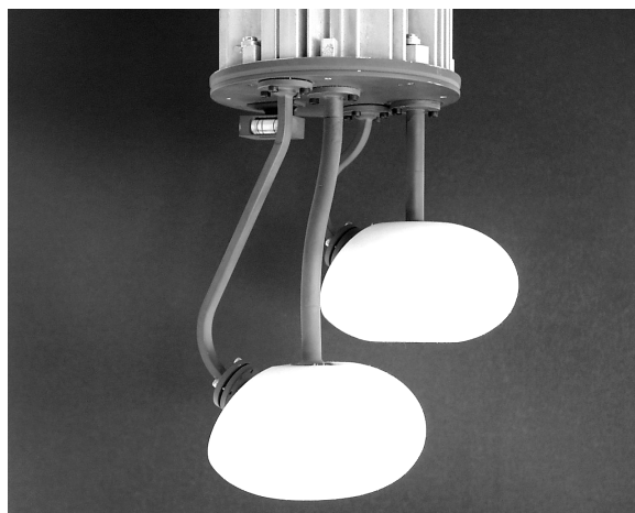
FIGURE 15.35 SAMBA base station lens antenna assembly for sectored cell coverage, 39.5 to 43.5 GHz, G = 19.5 dBi.
