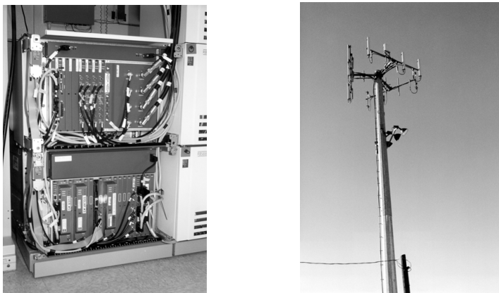
FIGURE 24.16 Prototype adaptive antenna base station equipment (DMAD = DAMPS minimal array downlink) for TDMA (IS-136) 1900-MHz PCS-band deployed in commercial traffic. The size of the physical array antenna enclosure is 66 \times 44 cm (height \times width).
