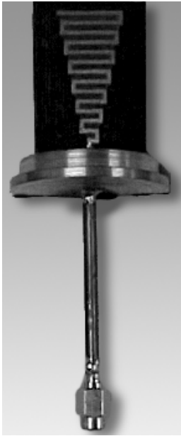
FIGURE 12.43 The prototype of taper meander line with e_1 = 2 mm and e_2 starting from 3 mm and ending with 17 mm on a 29-mm dielectric slab. (From ACES J. , 15(3), 159, 2000.)
