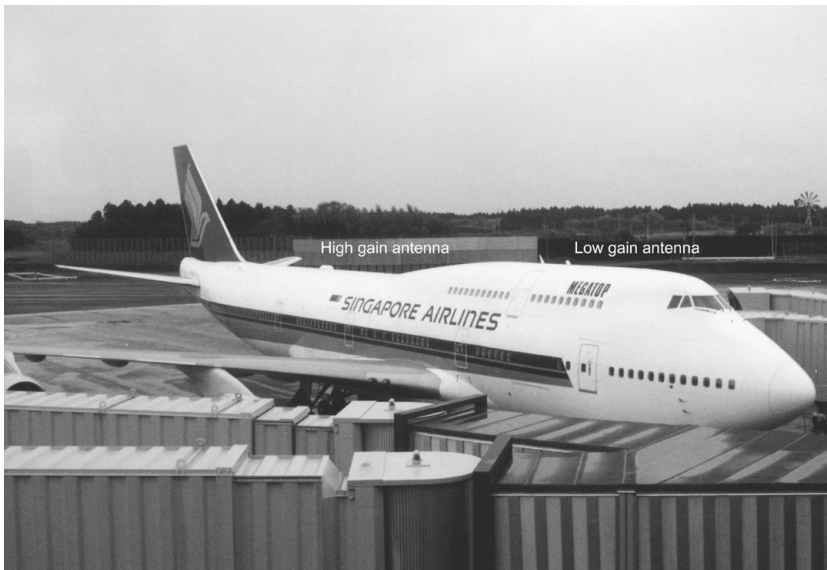
FIGURE 13.15 Photograph of low-gain and top-mount high-gain antennas installed on a Boeing 747.
