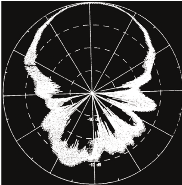
FIGURE 6.19 Typical axial ratio plot of synchronous subarray of microstrip patch antennas.
