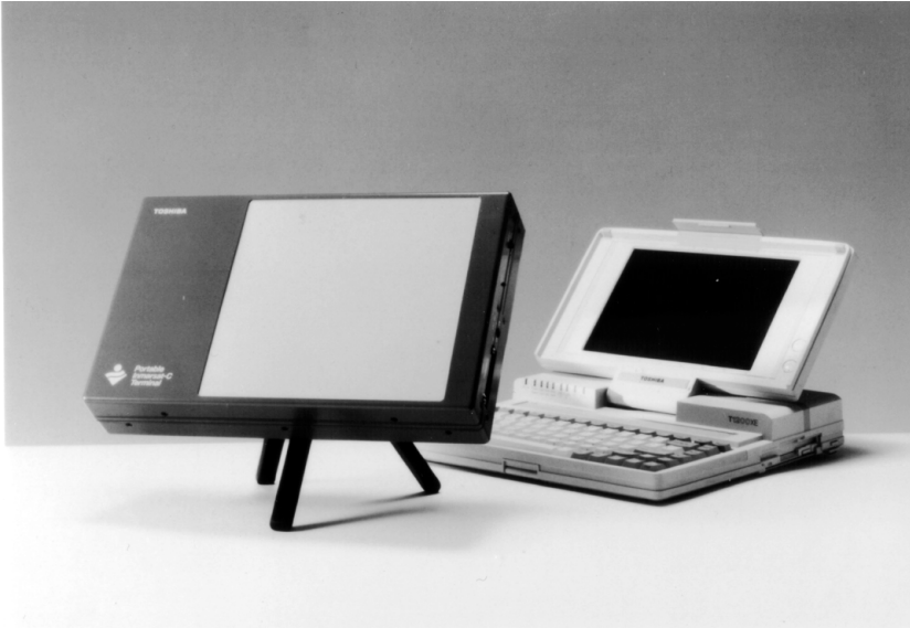
FIGURE 13.21 Hand-carried INMARSAT-C earth station. A receiver with a flat antenna weighs about 4 kg and has a compact size (320-mm weight \times 210-mm height \times 62-mm depth). (Courtesy of Toshiba.)
