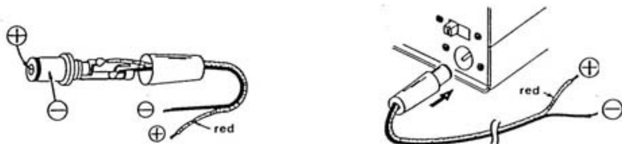
Figure 4-2: Plugging in external power to charge NiCad batteries.
