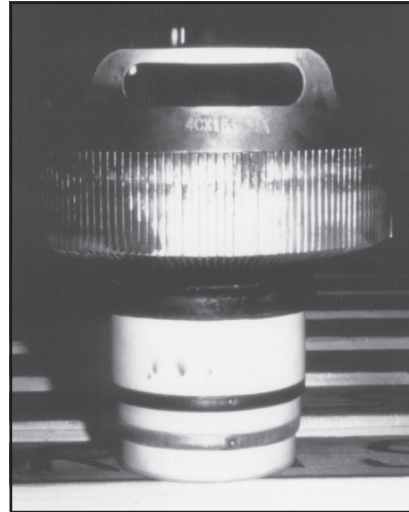
Figure 9.20 A 4CX15000A tube showing signs of external arcing. (Courtesy of Econco.)
