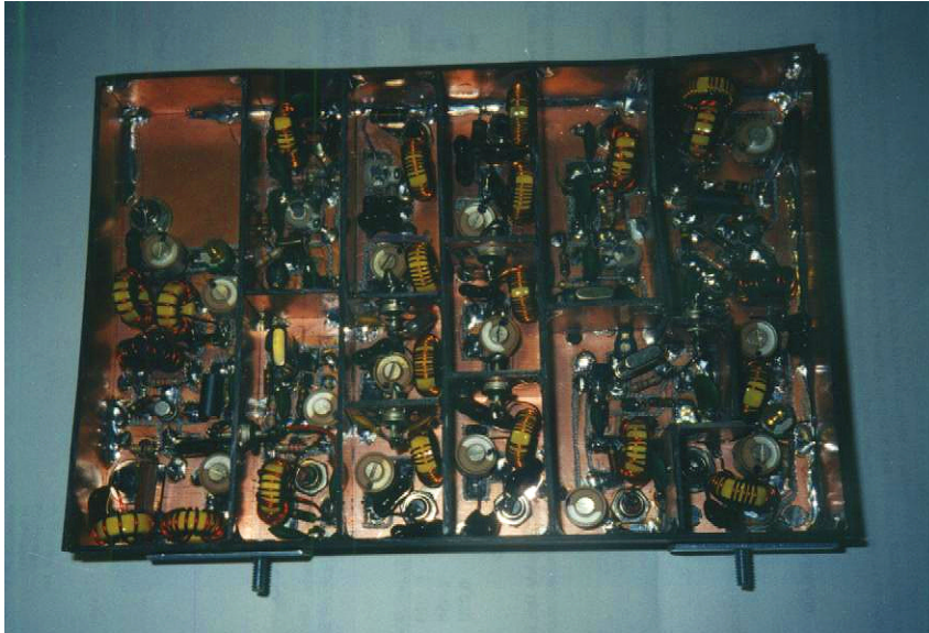
Converter modules for 20 meters, 30 meters, 40 meters, and 12 meters
