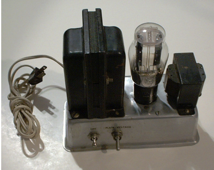
A power supply made from parts salvaged from an ancient radio.
