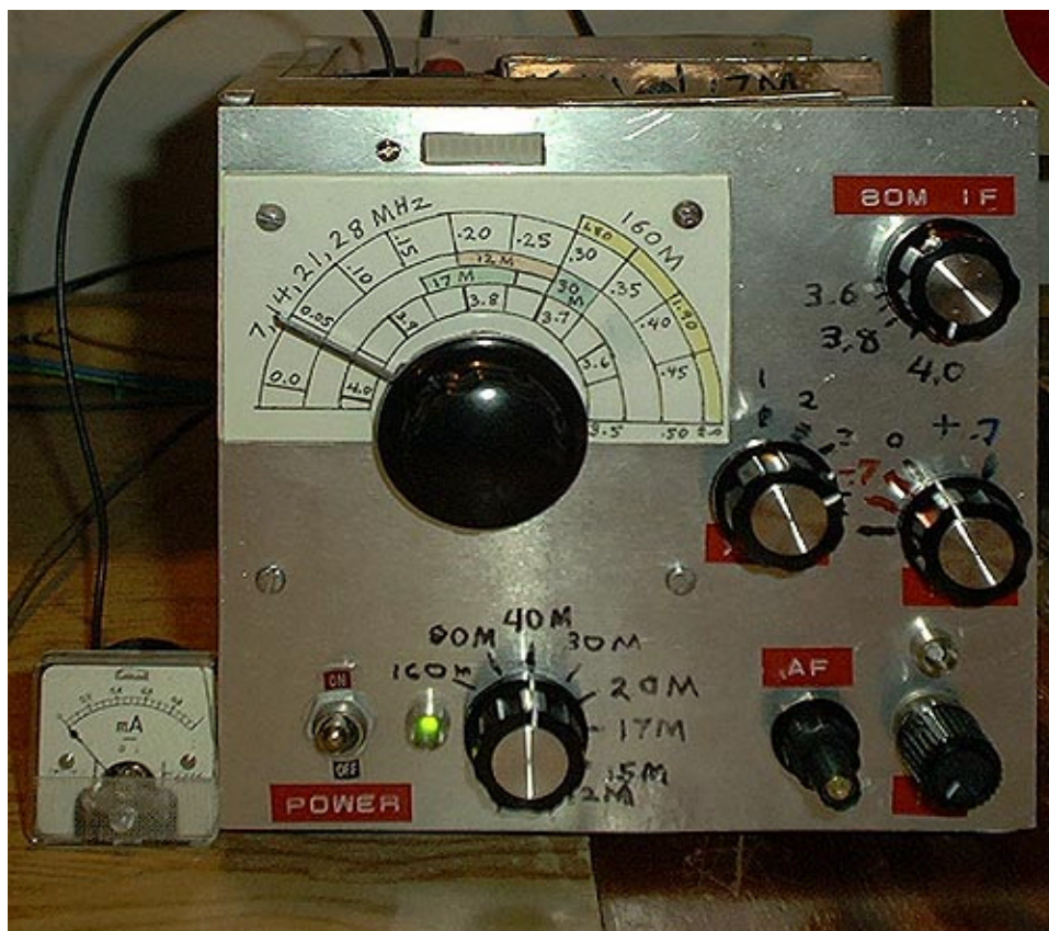
Homebuilt all-band dual conversion HF ham receiver.
