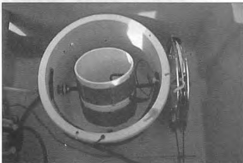
Fig 4.16: A variometer made by GW4ALG. The fixed coil is wound on a plastic bucket and the inner moving coil is wound on a section of plastic pipe. The spindle is turned from a section of wooden dowel.
