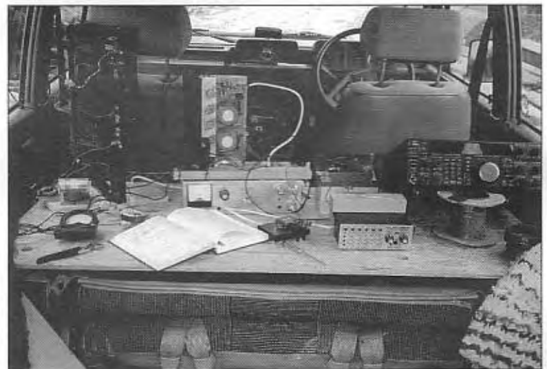
Fig 1.17: Operating position inside the vehicle. The variometer and matching transformer components shown strewn around the 'desk' on the right; part of the attempt to tune and match the antenna.
