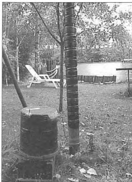
Fig 4.11: General view of the lower section of the helical antenna. The winding packets can be clearly seen. The plastic waste-paper basket loading coil can be seen in the foreground.
