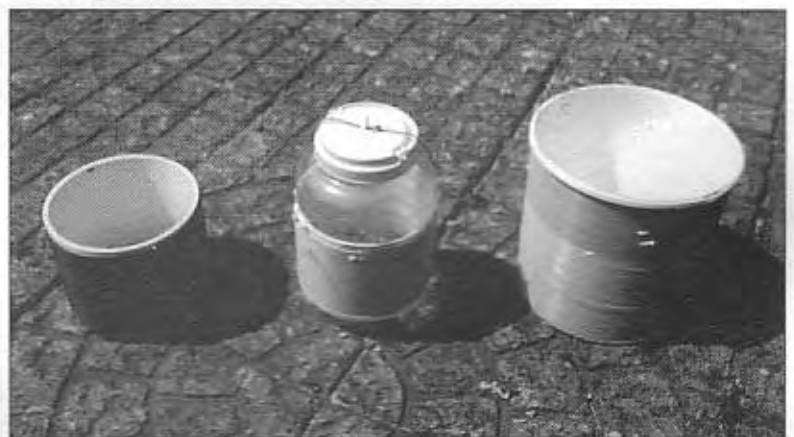
Fig 4.14: Three examples of loading coils by G3KAU. On the left the coil former is a large diameter plastic pipe. The centre coil is wound on a plastic rice container while the one on the right is wound on a plastic bucket. (Photo 14)
