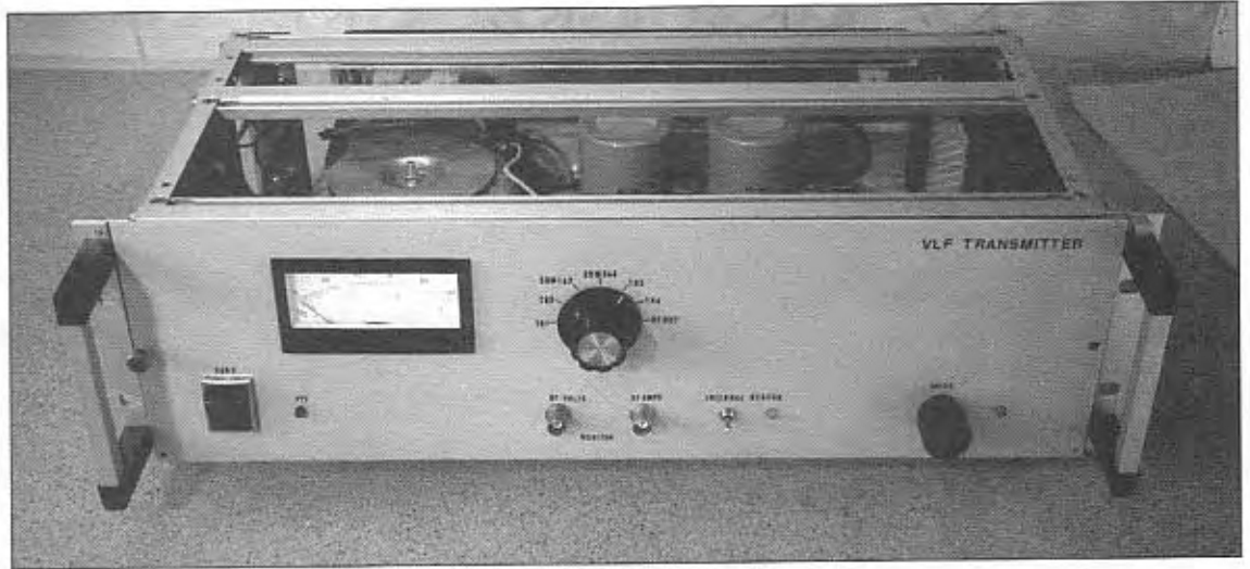
(left): 1kW Class D transmitter built by Lech, G3KAU. This design uses the original GOMRF board with some modification.
