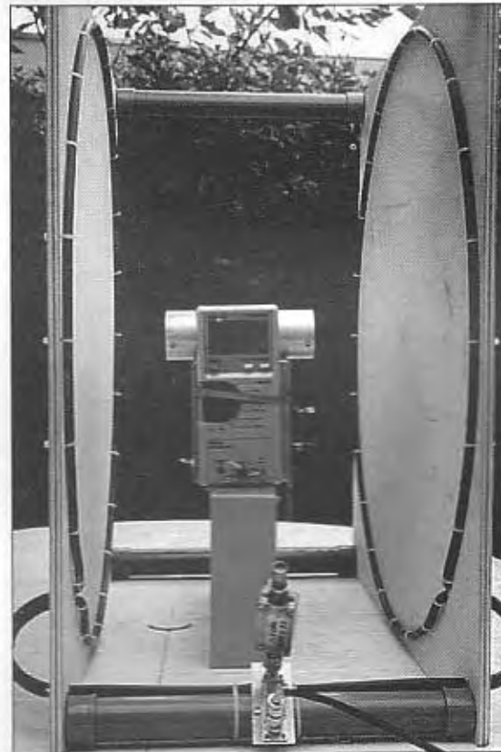
Fig 6.10: Field strength meter calibration arrangement using Helmholtz coils.
