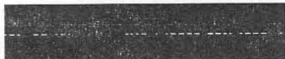
The signal from G0MRF, as seen by VE1ZJ, using Spectrogram. The parallel lines are sidebands of the Loran navigation system.
