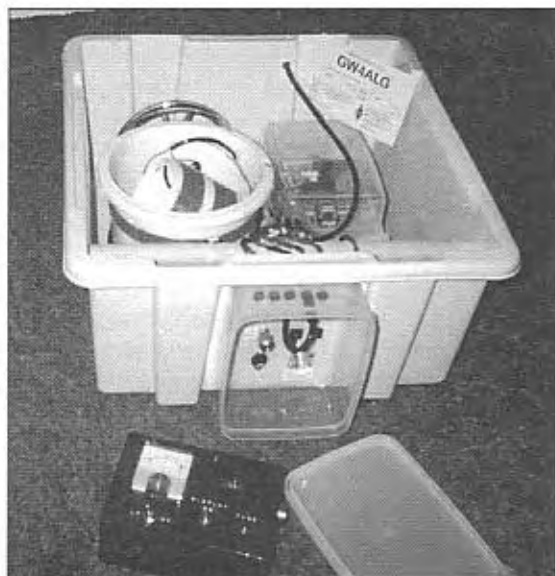
Gift-wrapped. The GW4ALG loading coil with weather protection.
