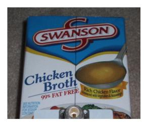
Place the probe point-down on the Brik, with the point passing through the 5/8" hole you cut in the front face of the Brik. Center the N connector body on the line you drew on the Brik. Take a marker and mark the four mounting holes onto the Brik, as shown at left. Placing a mailing label on the Brik (as I show here) helps to make the marked points more visible.
