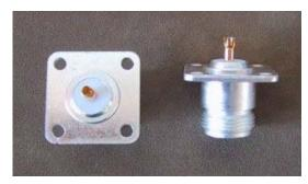
The probe consists of a male N coaxial connector with a short length of #12 or #14 copper wire soldered into its "solder pot." At left is a photo of a pair of silver-plated N connectors, which I purchased from Fleeman, Anderson, & Bird. Nickel-plated N connectors can be had for less, but they may not be "microwave-friendly" due to lossy insulation material. Go for silver. Be
