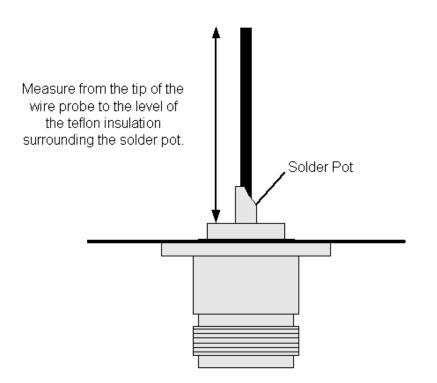
The touchiest measurement in the whole Tetra Brik antenna project is the length of the wire in the probe assembly. The length is the free-space wavelength divided by four. For Channel 6, that would be 123.1 millimeters divided by 4, or 30.77 mm. Now, the idea here is to do your best. Admittedly, measuring a fraction of a millimeter is a dicey business, and although the closer you come, the more sensitive your antenna will be on Channel 6.
