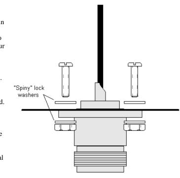
well, the Brik's foil liner must contact the N connector body!
