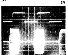
Fig 3—CW-keying waveforms for the TS-850S in the semi-break-in mode (A) and the full-break-in mode (B). The upper traces are the actual key closures; the lower traces are the RF envelopes. Horizontal divisions are 20 ms. The transceiver was being operated at 100 W output on 14.02 MHz. Other than a somewhat hard first keyed element (in both VOX and full-break-in modes), the TS-850S's CW keying shaping is excellent.
