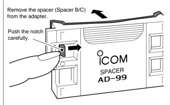
Push the notch carefully with your finger to remove the spacer (Spacer B/C) from the adapter (Spacer A).
