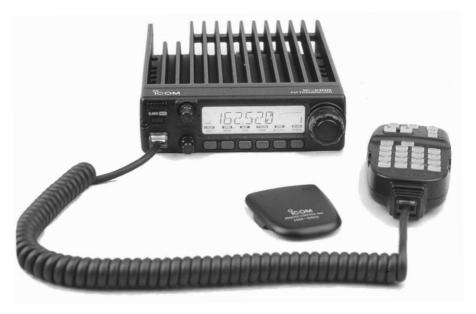
well. Like its predecessor, the IC-2000H, the '2100 has a large easy-to-read display and offers the ability to tag memories with up to 6 alphanumeric characters, a very handy feature for identifying both ham and public service frequencies.
