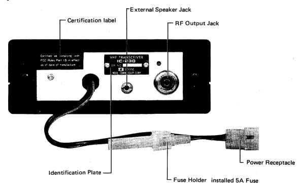
Power Receptacle: mates with DC cord plug supplied. Identification Plate: states model, serial number and date of manufacture.
