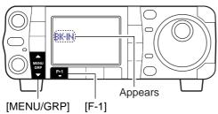
When using a paddle, set "Key Speed" in the quick set mode to adjust the keying speed. (p. 122)
