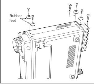
② Attach the MB-106 to the left side of the transceiver as shown below.
