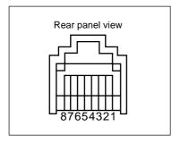
**CAUTION: DO NOT** short pin 1 to ground as this can damage the internal 8 V regulator.
