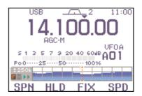
**NOTE:** If there is a lot of signal noise, turn the preamp OFF and the attenuator ON (p. 72) to reduce the input level and improve the readability of the scope.
