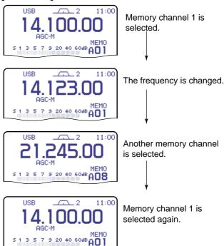
Changed frequency (14.123 MHz) does not appear and memorized frequency (14.100 MHz) appears instead.
