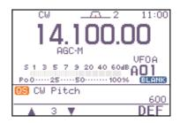
•This shows the default setting for the CW pitch control (600 Hz).
