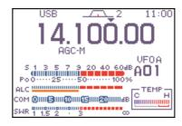
The multi-function meter also displays the internal temperature meter.
