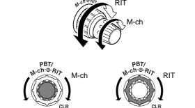
•When the RIT or ⊿TX function is ON, push and hold [F-1 RIT] or [F-2 ⊿TX] for 1 sec. to add or subtract the frequency shift to the display frequency.
