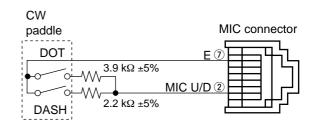
**NOTE:** The HM-103 can be operate as a CW paddle from both of the front panel and rear panel mic connector. But the HM-103 is not available the squeeze operation.
