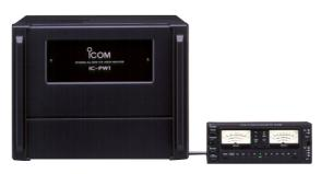
Full-duty 1 kW linear amplifier including an automatic antenna tuner. Has automatic tuning and band selection capability. Full break-in (QSK) operation is possible. The amplifier/power supply unit and the remote control unit are separated. An optional OPC-599 is required for connection.
