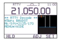
The transceiver has an RTTY decoder for Baudot (mark freq.: 2125 Hz, shift freq.: 170 Hz, 45 bps).
