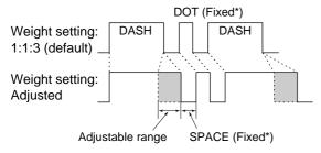
\*SPACE and DOT length can be adjusted with "Key Speed" only in the quick set mode.
