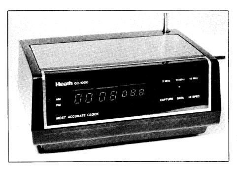
tion. The position of the digit in the code determines whether the digit represents an hour, a minute or a second. Time-code pulses are sent once each second, so that in the one-minute time frame enough information is sent to convey current hour, minute, second and day of the year.<sup>1</sup> Using this mechanism, the GC-1000 automatically calibrates itself to NBS.
