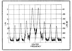
Fig 4—Spectral display of the IC-735 output during transmitter two-tone intermodulation distortion (IMD) test. Third-order products are 33 dB below PEP, and fifth-order products are 39 dB down. Vertical divisions are each 10 dB; horizontal divisions are each 1 kHz. The IC-735 was being operated at rated input power on the 20-meter band.
