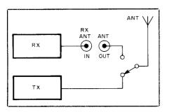
Fig 1—Antenna TR connections for the IC-735. RX ANT IN and ANT OUT are connected by a jumper for normal operation. An external preamplifier connected in place of the jumper needs no TRswitching provisions. An external receiver is controlled by the IC-735 TR circuitry when it is connected to the ANT OUT jack.
