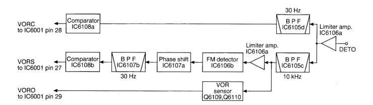
The signal from the AM detector (DETO) is buffer amplified at the VOR amplifier (IC6105b).
