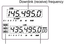
Satellite mode indication Uplink (transmit) frequency
