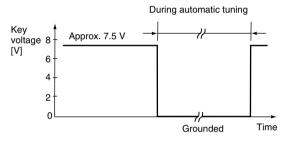
If the key voltage is more than 8 V, switch the mode switch (S1) to OFF mode (lower position).
