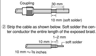
(3) Slide the connector body over the cable and solder as shown below.
