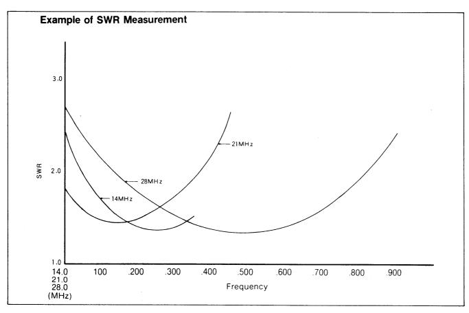
Suppose a typical tribander antenna covering 14MHz, 21MHz and 28MHz has VSWR values as shown in the diagram.
