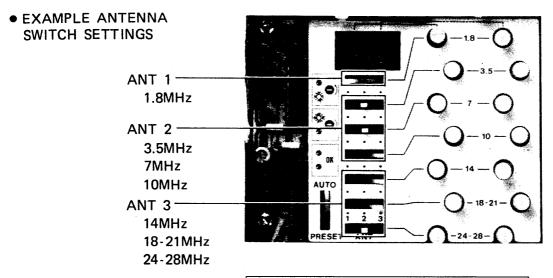
NOTE: The switches are set for operation with the antenna system shown.
