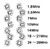
Approximate positions of the PRESET controls for 50  $\Omega$  antenna systems.
