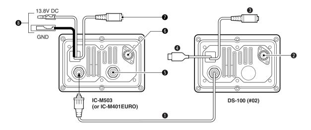
NOTE: Binding the GPS cable, GPS connector, clone receptacle, antenna connector with water-resistant tape, increases the waterproofing of the controller.
