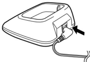
**3** Slide the battery pack or a transceiver with a battery pack into the charger.
