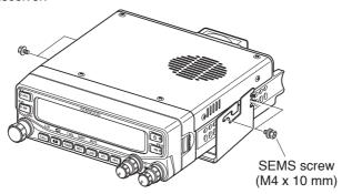
Set an appropriate angle for the main unit, using the 3 screw slots on the rear edge of each bracket side.
