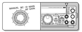
Depending on the type and gain of your antenna, and the condition of the band, you may also prefer leaving the **MAIN RF** control turned counterclockwise by the same amount rather than turning it fully clockwise. When using FM mode, always set the **MAIN RF** control fully clockwise.
