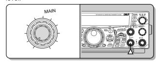
**Note:** The position of the **MAIN AF** control does not affect the volume of beeps caused by pressing keys nor the CW transmit sidetone. The audio level for Packet operation is also independent of the **MAIN AF** control setting.
