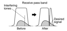
Press [A.N./ LEVEL] to toggle the Auto Notch Filter ON and OFF.
