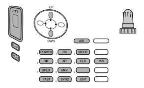
Each time you press the desired key, the Commander will automatically enter transmit mode and send the corresponding control command to the TS-2000 (Transporter).
