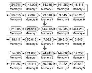
You can store data in the Quick Memory only when using VFO frequencies for both transmitting and receiving.
