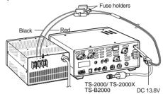
First, connect the DC power cable to the regulated DC power supply; the red lead to the positive terminal and the black lead to the negative terminal. Next, connect the DC power cable to the transceiver's DC power connector. Press the connectors firmly together until the locking tab clicks.
