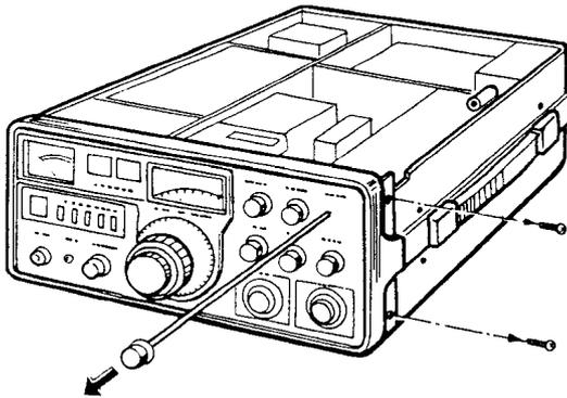
1. Draw out FINAL shaft. (Do not remove the knob mounted on the coupling showing up on the side of BPF case.)
