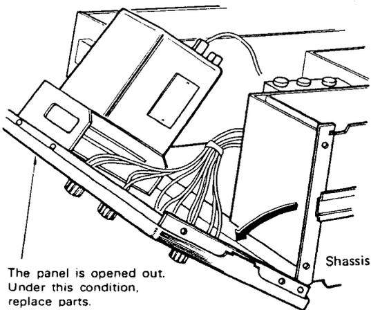
3. The panel is opened out. Under this condition, replace parts.
