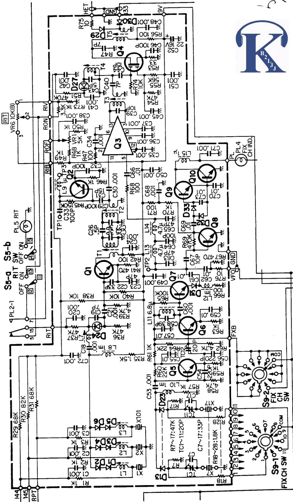
Q1: 25C388A, Q2, 8: 25C460(B), Q3: SN76514N, Q4: 3SK41(L), Q5~7: 25C458(B), Q9: 25C733(Y), Q10: 25C735(Y), D1~6, 13~23, 29, 30: 1S1555, D24, 27: 1S2208, D31~33: 1N60
