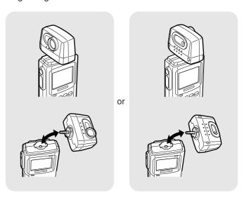
To reinstall the camera unit, first position the port on the camera unit over the port on the main unit so that the two units cross at right angles.
