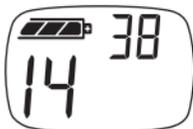
T5320 will have the Channel 1-14 on display. Model T5410 and T5420 display includes the Interference Eliminator Code (0-38) as well as the Channel.
