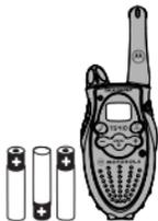
Turn it off and remove batteries.
