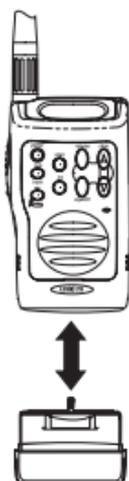
2. Use a quarter to turn the screw that connects the battery pack to the HH940. Be sure the battery pack fits tightly against the HH940's body.
