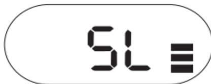
Press and hold ▲ on the **chan** button to adjust the “squelch gate” so high that no signals get through.
