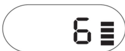
2. The channels flash on the LCD display as the HH940 looks for a transmission.
