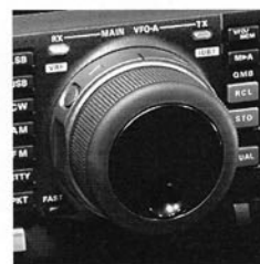
VRF and IDBT Switches are located on Shuttle Jog Dial for ease of operation.
