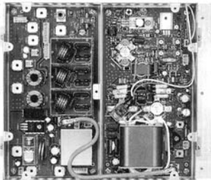
● FTV-1000 Power Amplifier Left : Low-Pass Filter Right : PA Module
