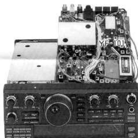
SSB Filter Location (replacing Ceramic Filter)
