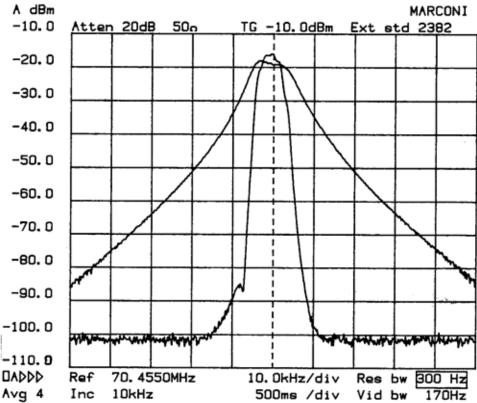
The result of the bandwidth improvement shown above is the reduction of close in intermodulation from multiple signals. The IMD dynamic range will be improved by more than 10 dB for some tone spacings. The blocking dynamic range will be improved by 20 dB or more for some signal spacings. The main
