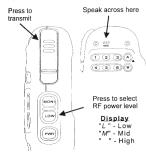
To transmit, press and hold the PTT while speaking across the microphone element grill in a normal voice. Release the PTT to receive again. During transmission, LCD bargraph segments appear and the red TX lamp just above the DIAL knob turns on (as shown in the graphic).
