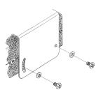
□ Position the transceiver in the bracket so that the holes in the side are aligned with those in the bracket, and bolt the transceiver into place using the supplied short screws and flat washers. The FS-10 Smart Controller hanger may be installed wherever convenient.
