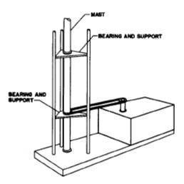
The mast may also be held in a bearing as shown above and the rotator housed outside the tower. The rotator drives the mast by using two sprocket gears and a chain. This requires two identical #50 sprocket gears and a length of #50 roller chain.
