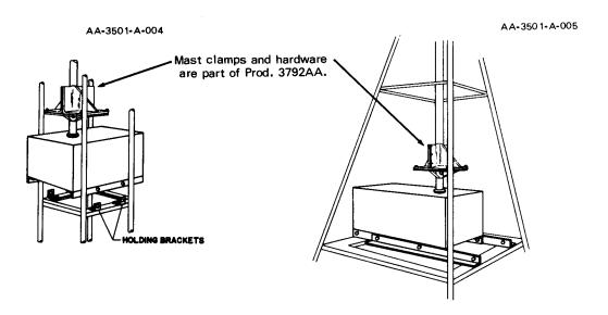
4. On top of large towers. Where a large, flat-topped tower is available, the rotator may be installed directly on top. This may be secured by bolting directly and securing the four corners with four angles supports to the legs of the tower as shown in the illustration.
