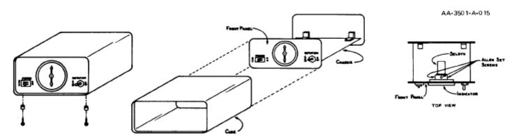
The indicator dial will usually require slight adjustment for accurate readings. Remove the chassis as shown above. Loosen the three Allen screws in the dial frame holding the selsyn and carefully rotate the selsyn in the frame until the dial indicates the proper direction. Tighten the Allen screws and replace the cabinet. **CAUTION**
