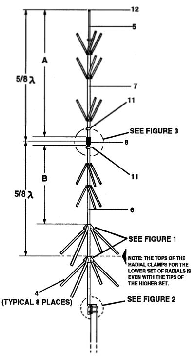
Figure 4 Overall View-VHF Dimensions
