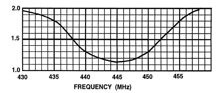
Figure 8 Typical VSWR **Curves with Antenna Set for 146 and** 445 MHz.
