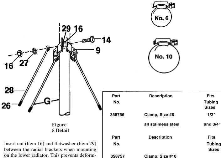
on the lower radiator. This prevents deforming the brackets when fully compressed. The brackets should be tightened enough so that the UHF radials do not twist on the bolt.
