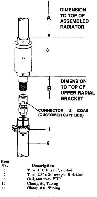
Figure 3 Upper Radiator/Coil Assembly NOTE: At 14 MHz, A = 45" (1143 mm), B = 23 1/2" 597 mm).
